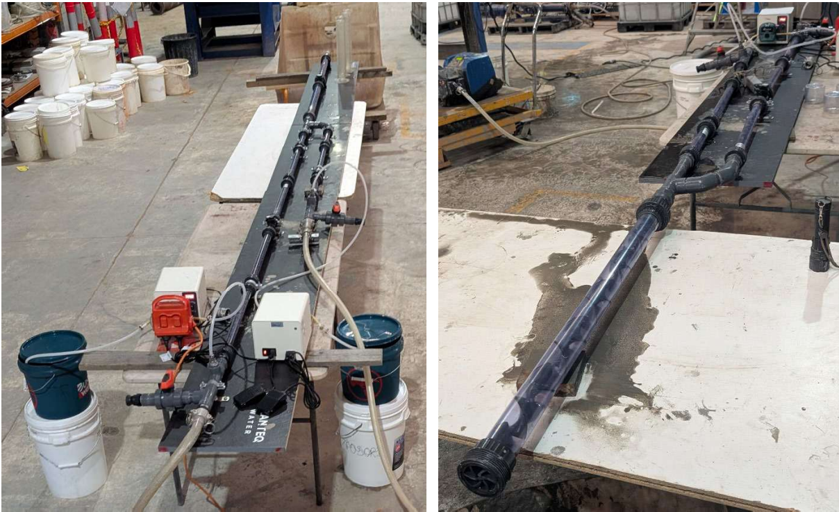
Figure 5 Static mixer rig set up
