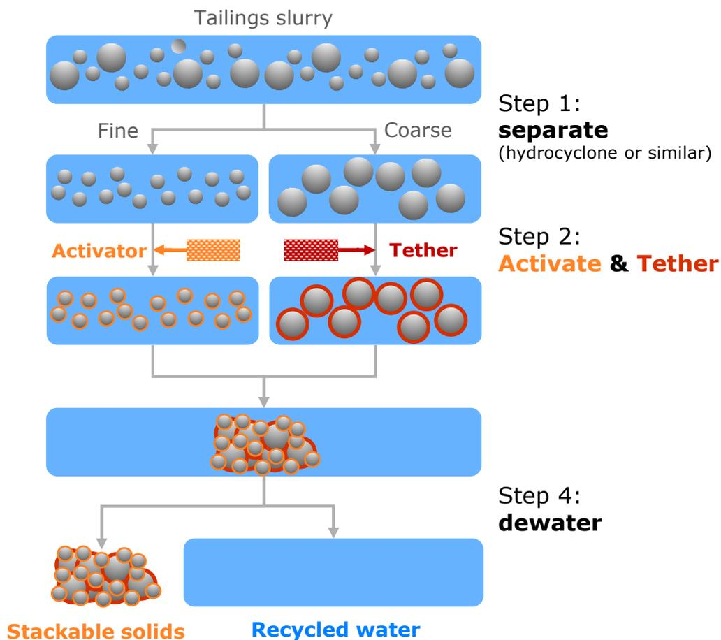
Figure 1 Schematic of ATA process
