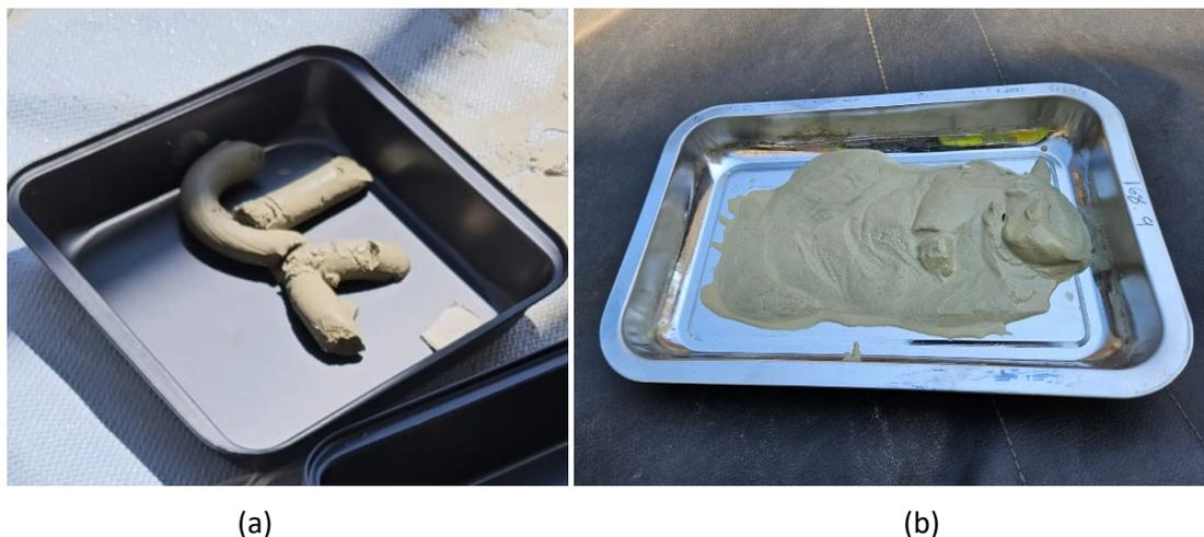
**Figure 15 Core samples taken from the geotextile bag after 24 hours of dewatering for (a) ATA treated and (b) untreated tailings**
