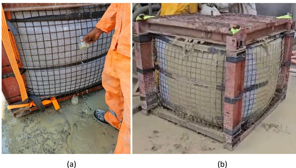
**Figure 16 Fines losses during filling of geotextile bag, comparing (a) ATA treated and (b) untreated tailings**
