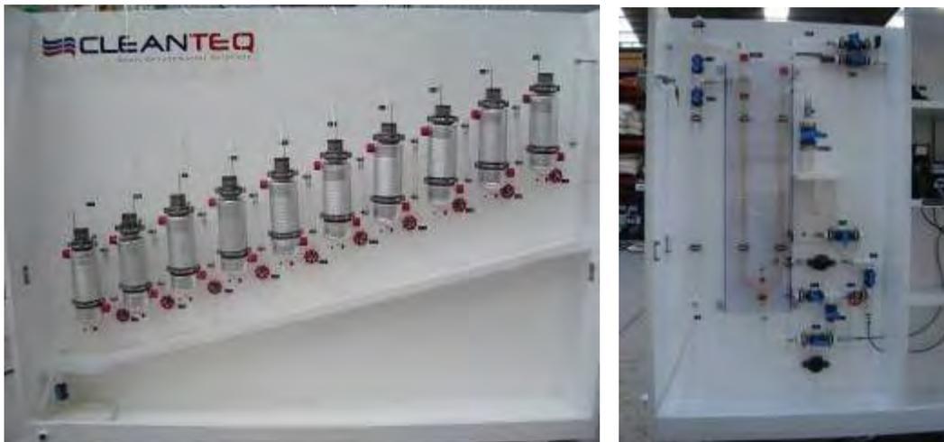
**Figure 9: Sorption and Desorption Mini pilot plant for uranium**
